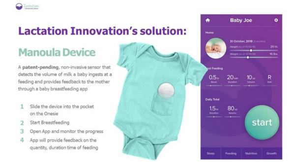
The Manoula device is a non-invasive sensor that uses proven safe technology to accurately detect the volume of milk an infant ingests during breast feeding. The device slides easily into a pocket in a customized onesie worn by the infant and transmits the data via Bluetooth technology.
